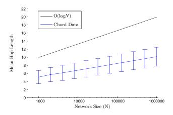
Fig. 4. Chord baseline validation for mean hop length. The plot of  $O(\log N)$  is the expected upper bound for the mean hop length in a pure Chord system. The results obtained via experiments fall below the upper bound, partially validating the RC-Chord protocol.
