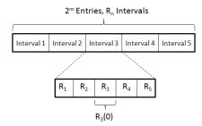
Fig. 3. Example agent mapping for a cluster with m bits of address width, and n resources. The  $2^m$  address entries are divided into  $R_n$  intervals. Each interval has one entry for each of the n resources. The initial interval for resource three is shown as  $R_3(0)$ , being the first entry for resource three in interval three.
