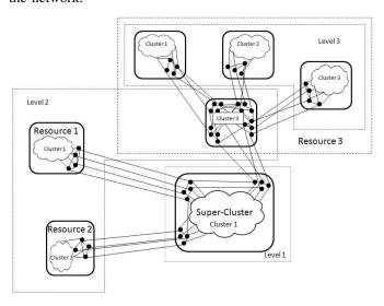
Fig. 1. An example RC-Chord instance with three levels. The super-cluster exists as the sole level one cluster. Its nodes serve as super peers for level two clusters, with a single level-two cluster for each resource. Clusters at level two begin the formal sub-graph for each resource type, and may extend into additional levels based on number of nodes for each resource.
