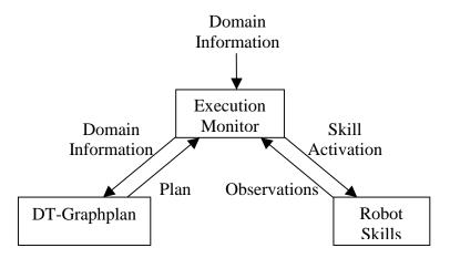
Figure 1. The DTRC Robot Architecture.
