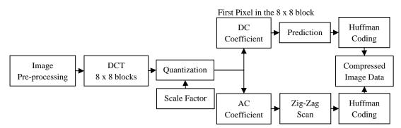
Fig. 1. Block Diagrams of Sequential JPEG Encoder
