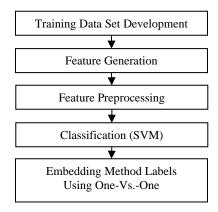
Fig. 4. Block Diagrams of Multi-Class Detection System
